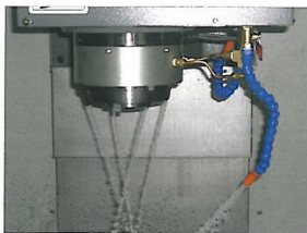
Coolant Jets Around Spindle (Opt.)
