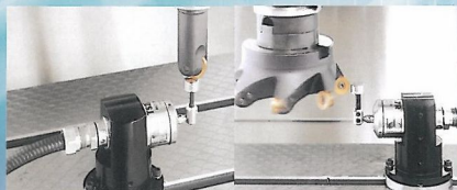
6. AUTOMATIC TOOL LENGTH & RADIUS MEASUREMENT (RENISHAW TS-27R)
