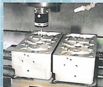
7. WORKPIECE PROBE (RENISHAW MP-10/12)
