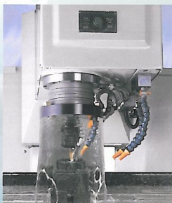
2. GRAPHITE CUTTING WATER CURTAIN DEVICE.
