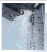
The splash nozzles surround the spindle and they offer large coolant water to the right cutting area. The splash coolant takes away heat from tool and workpiece to increase the cutting accuracy.
