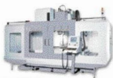
Vertical machine center 400MM ~ 3200MM X axis travel
