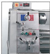
▲ Variable-speed change 2 steps speeds
