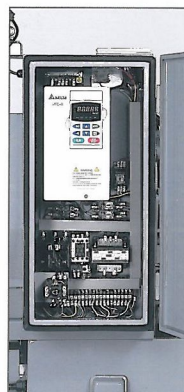
▲ Electrical box for Variable - speed change Lathe
