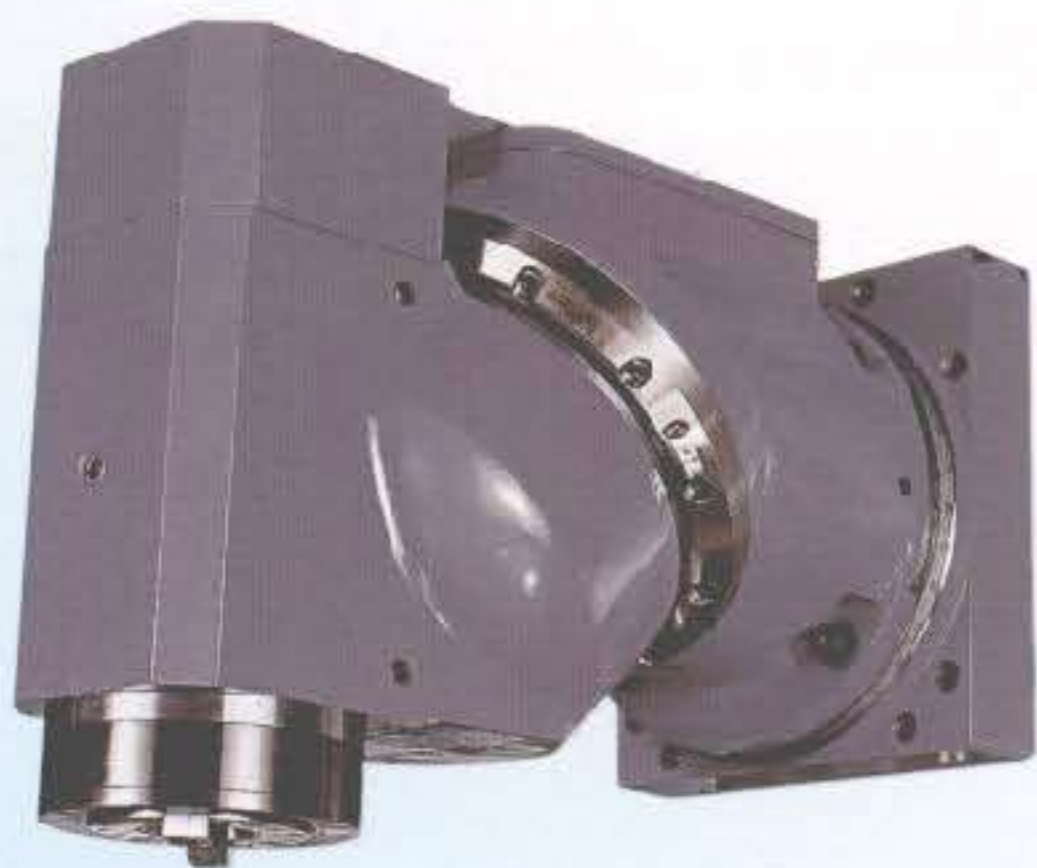
1. MODEL VH-2 AUTOMATIC 2 POSITIONS MILLING HEAD: 3500 rpm.sk50 Taper,25kw Motor,750Nm Torque • NECK : Manual 360° Indexing • 45° PLANE : automatic Vertical & Horizontal (0/180 Deg)
