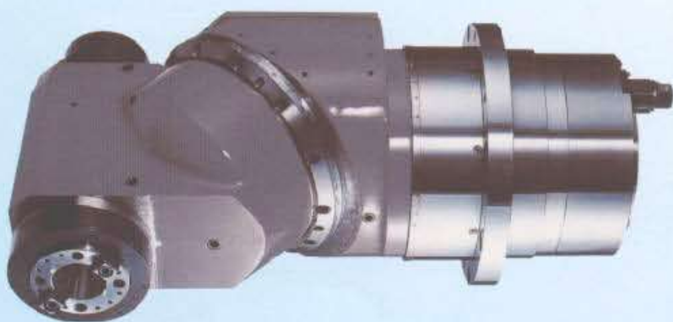
3. MODEL VH-5 AUTOMATIC 5 INDEX MILLING HEAD: 3500 rpm.sk50 Taper,25kw Motor,750Nm Torque • NECK : automatic 5° Indexing • 45° PLANE : automatic 5° Indexing
