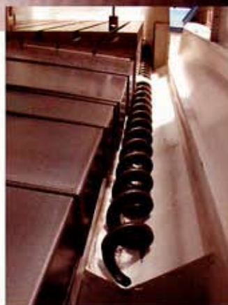
Dual coil chips conveyor (STD)
