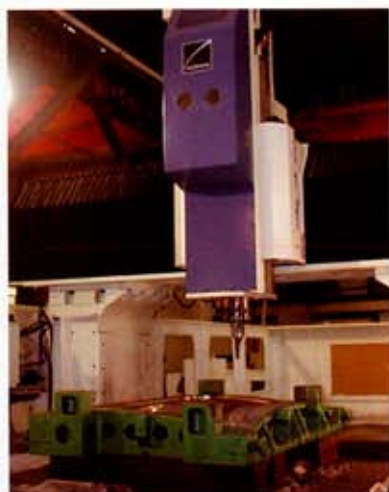
Machining of sheet metal mold
