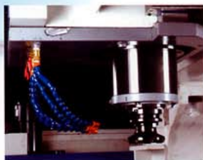
Spindle head and coolant nozzle ring
